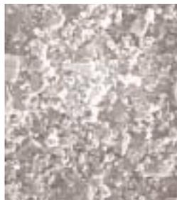
*Pressed Carbon Block Magnified 1,000 Times*
