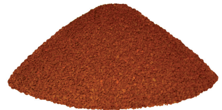
Example of Bayoxide® E33 Granular Ferric Oxide Media
